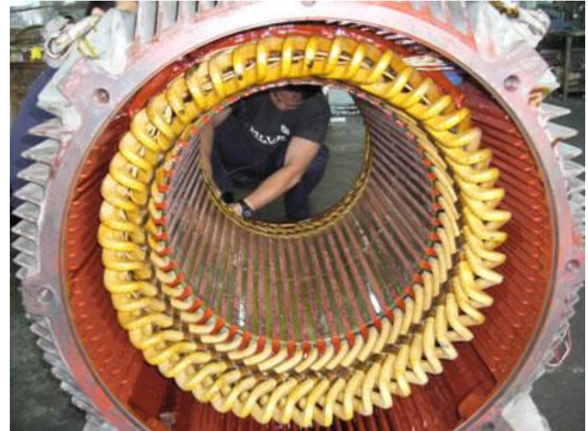
Stator Winding of MW HV Induction Motor
