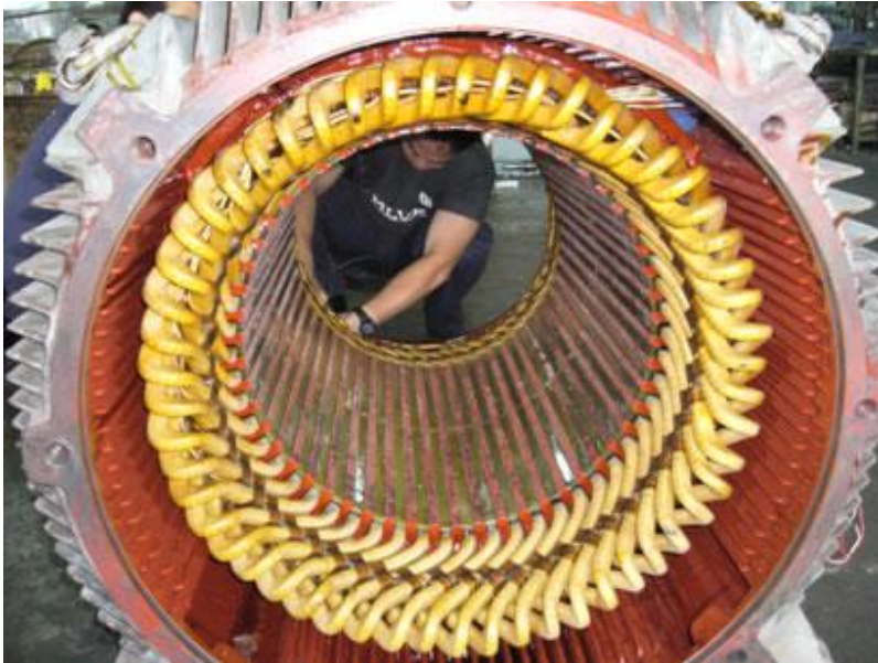
Stator Winding
