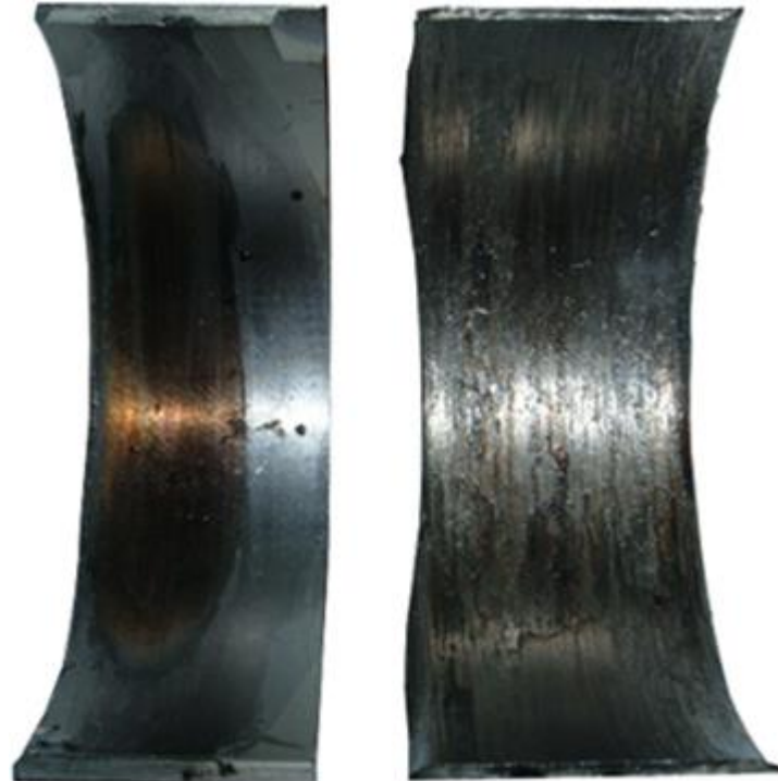
Bearing failure due to oil starvation
