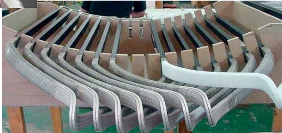
Stator Winding Construction
